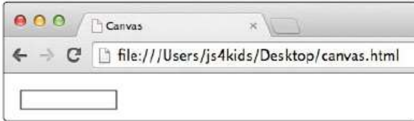
Figure 13-4: Using strokeRect to draw the outline of a rectangle
