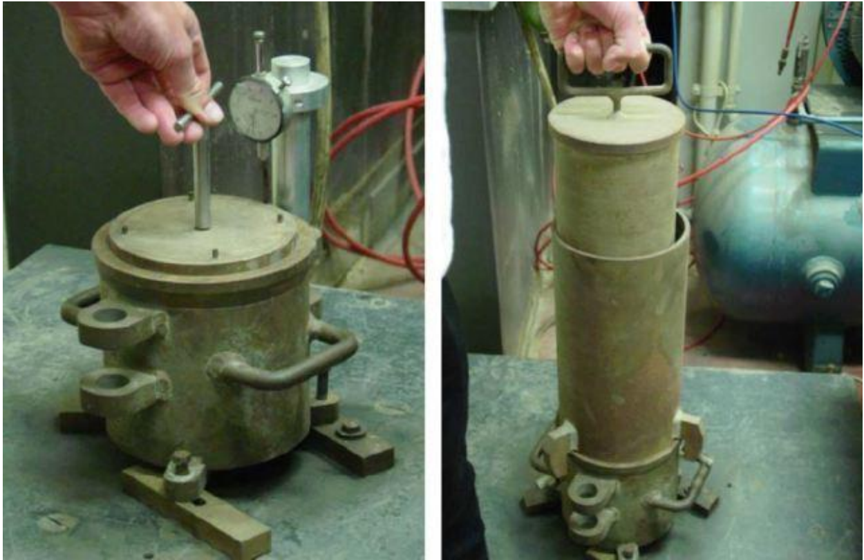
Fig-2 Relative density test of sand
