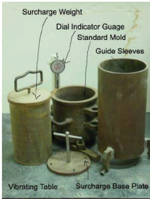
Fig-1 (Relative density test apparatus)
