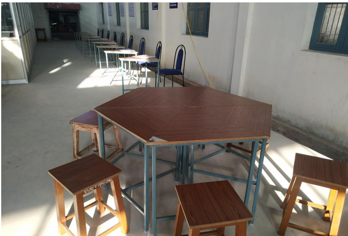
Multipurpose Working Table. Table size 0.762mts side equilateral Triangle Top and 0.762mts Height.
