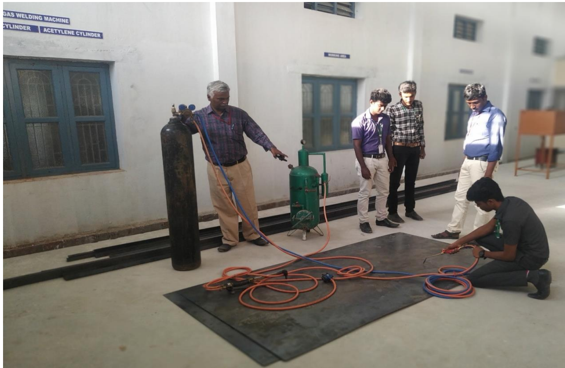
Setting Pressure of the Oxygen and Acetylene cylinder to cut the plate by Gas welding Machine
