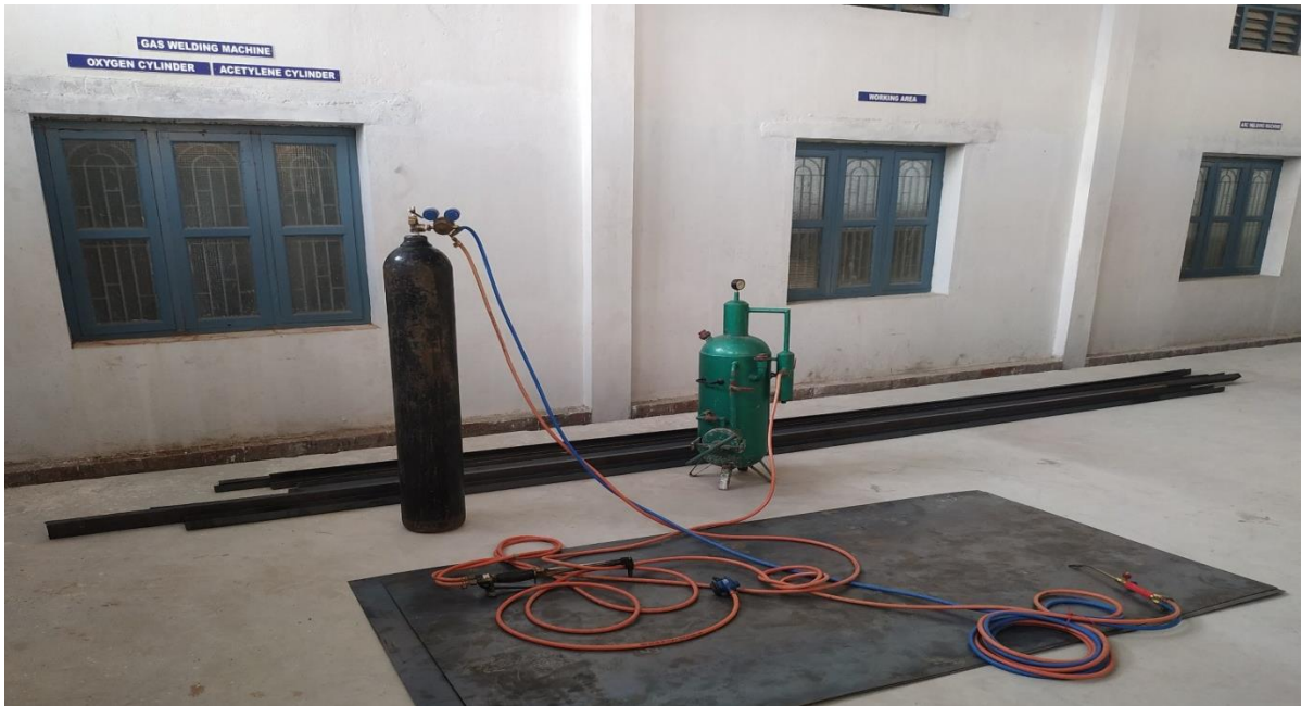
Oxy acetylene Gas welding Machine This Machine has the facility to Weld and cutting the plates.
