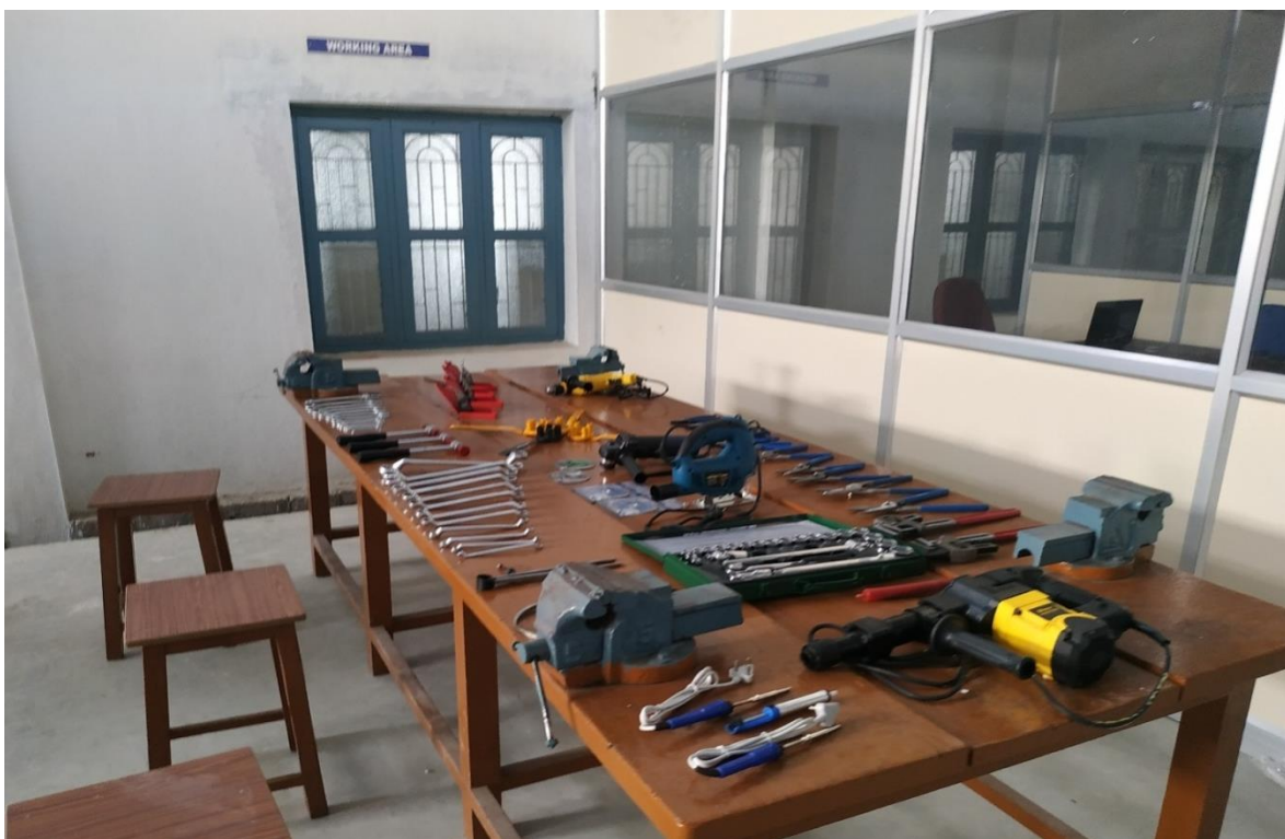
Tools available in this Lab: Double Ended Spanner Set, Ring Spanner Set, Clutch Spanner, Allen key set (Black), Pipe Wrenge, Box Spanner, Round, Triangular and Square files, Cutting Plier, Screw Driver Set, HOT air gun, Soft faced hammer, Lever Hacksaw frame, Welding accessories ,Digital Multi Meter, Electronic Precision Screw Driver Set, Soldering Iron and De-Soldering gun.
