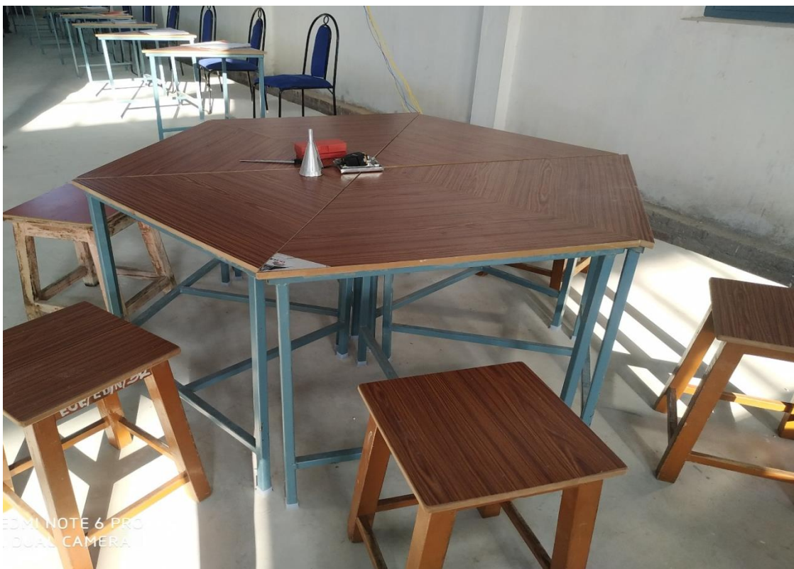
Multipurpose Working Table. Table size 0.762mts side equilateral Triangle Top and .762mts Height
