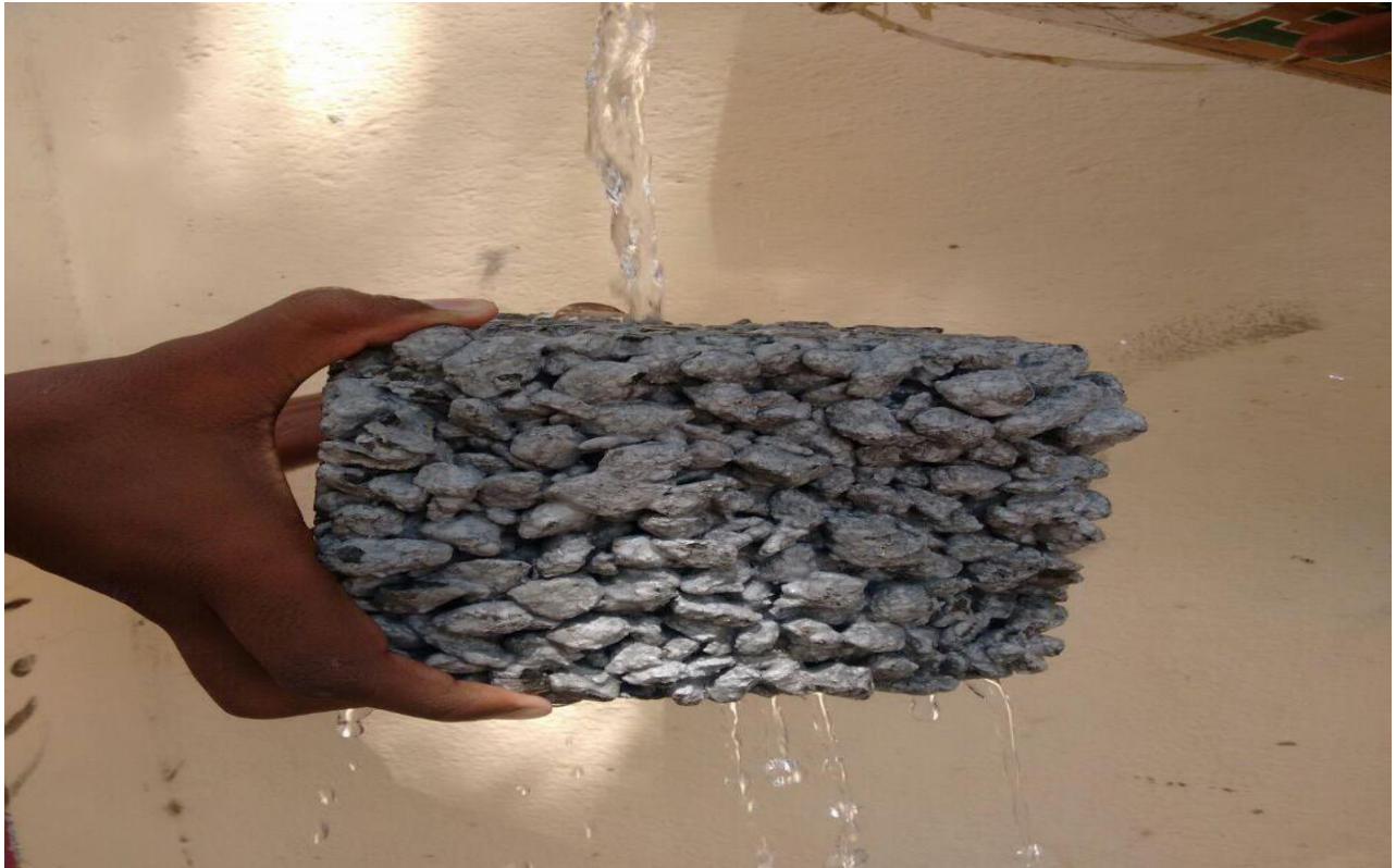
Demonstration on Performance of Pervious Concrete
